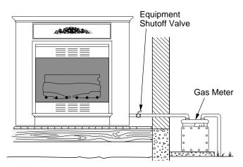
Figure 25 - Checking Gas Joints for Natural Gas Unit (Shown With Optional Mantel)
